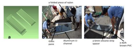
**Figure 1.** Showing top view of rhizobox diagram (a) and components of rhizobox (b)
